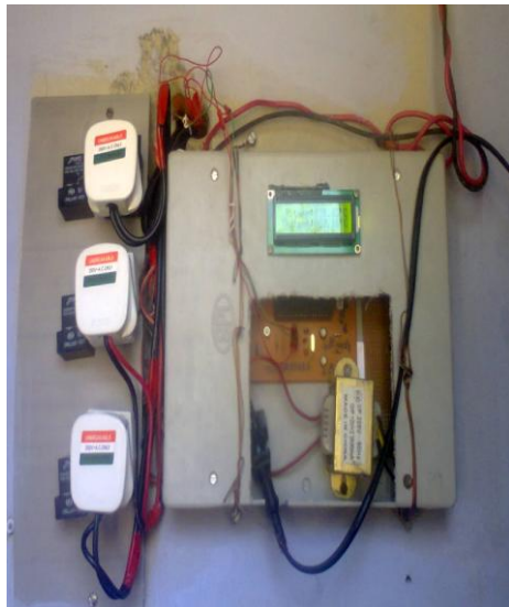
Figure 8: Control system with LCD & relay driver
